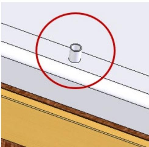
Install two high strength 3/8"-16 shouldered eyebolts (1200 pounds minimum capacity each) (not included) into weld nuts and tighten. (Refer to Figure 4):
