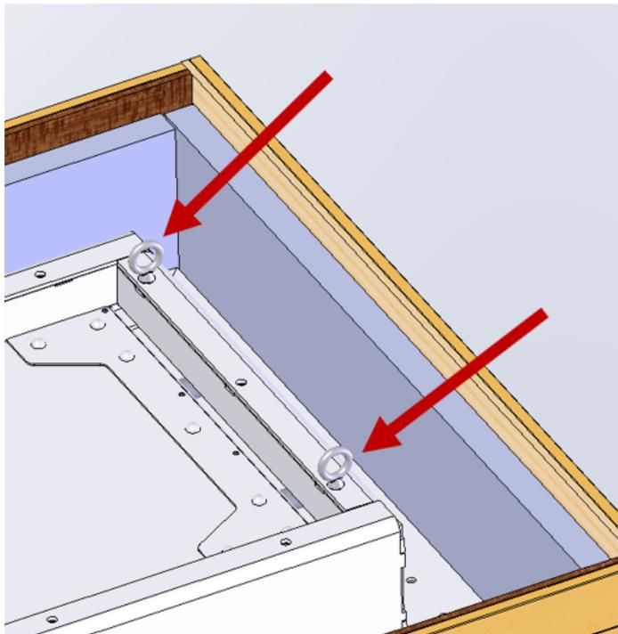
Attach two lifting straps or cables (1200 pounds minimum lifting capacity each) to eyebolts and lift vault door from shipping crate. (Refer to Figure 5):
